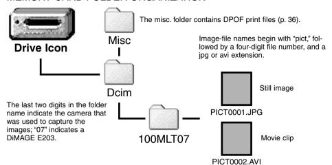
Once the camera is connected to the computer, image files can be accessed by simply double clicking on icons. Copying images can be done by dragging and dropping the image-file icon into a location in the computer. Never change image file names on the memory card or save data to the card using a computer; it may hinder camera operation and cause malfunctions. Never format the memory card from the computer; always use the camera to format the card.
