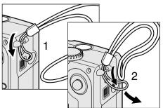
Pass the small loop through the strap eyelet on the body (1).
