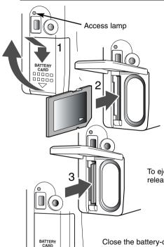
Open the battery-chamber door by sliding the door down (1) to release the safety catch; the door should spring open.
