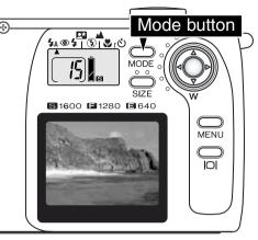
The mode button gives quick, easy access to the camera's flash modes and subject programs. By pressing the mode button, the mode indicators point to the active mode. To cycle through the modes in reverse order, press and hold the mode button and use the left key of the controller to change the modes. When the camera is turned off, the mode is reset to autoflash. The mode can also be reset to autoflash by pressing and holding the mode button for about two seconds.
