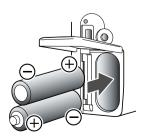
Although camera performance is better with lithium batteries, two AA-size alkaline or Ni-MH batteries can be used in this camera. The use of Ni-MH batteries are recommended over alkaline because of longer life.
