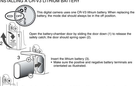
Close the battery-chamber door and slide it up (4) to engage the safety catch.
