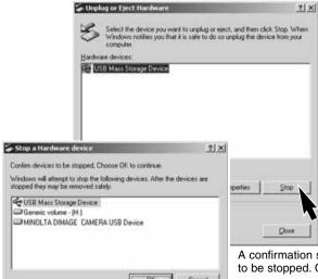
The hardware devices to be stopped will be displayed. Highlight the device by clicking on it then click "Stop."
