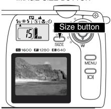
Changing image size affects the number of pixels in each image. The greater the image size, the larger the file size and the greater the pixel resolution. Choose image size based on the final use of the image – smaller images will be more suitable for web sites whereas larger sizes will produce higher quality prints.
