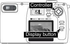
This camera is equipped with a zoom lens. The effect of the zoom is visible in the viewfinder and on the LCD monitor. To activate the LCD monitor, simply press and hold the display button.
