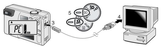
When the camera is properly connected to the computer, a drive icon will appear. Double click on the icon to access the camera's memory card; see page 45. If the computer does not recognize the camera, disconnect the camera and restart the computer. Repeat the connection procedure above.
