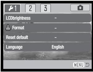
Navigating the menu is simple. Push the controller in the direction to move the cursor and change settings on the menu. Pressing the controller selects menu options and sets adjustments.
