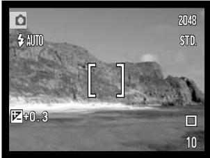
The exposure compensation must be set before the image is captured. When setting the exposure compensation, the amount of compensation is shown next to the exposure-compensation indicator on the monitor. When set to any value other than 0.0, the exposure-compensation indicator will be displayed on the LCD monitor as a warning.
