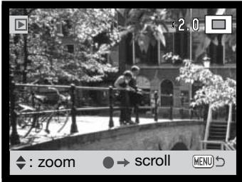
Moving the controller up increases the image magnification. Moving the controller down decreases the image magnification.
