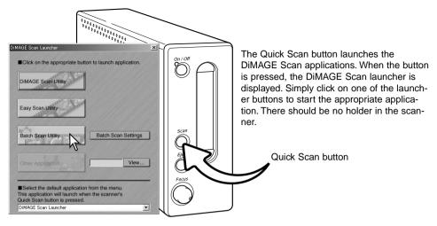
When the Batch Scan Utility button is clicked, the scanner will initialize. When the set-holder message appears, insert the holder into the scanner; all the frames in the holder will be scanned and saved, and the holder will be ejected automatically. To scan another batch, change the film in the holder and reinsert it into the scanner. Click the Batch Scan Utility button to begin scanning. The scanner only needs to be initialized before the first holder is scanned.
