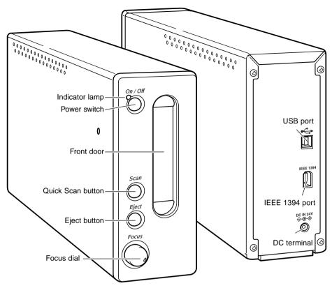
Do not use the focus dial until is has been activated in the DiMAGE Scan Utility's preferences dialog box. See the DiMAGE Scan software manual for details.
