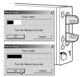
Turn the focus dial (1) until the black and white bars are at their longest extension. The black bar indicates the change in focus. The white bar indicates the longest extent of the black bar and the point of sharpest focus. Do not touch or hinder the holder.
