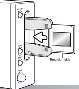
When the slide mount holder is in the scanner, the last slide can be removed and a new slide inserted without ejecting the holder. When replacing slide, take care not to change the holder position. A prescan should be made each time a slide is inserted; refer the DiMAGE Scan manual.
