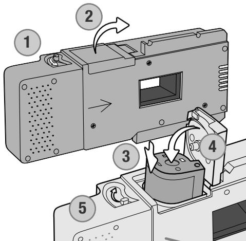
When the indicator lamp glows steadily, open the front door until the top of the door is aligned with the APS film-holder mark.
