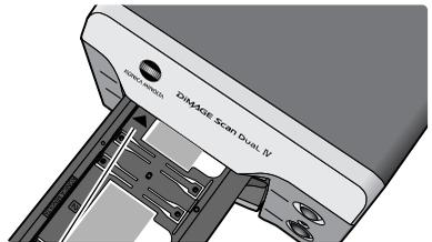
Carefully push the holder into the scanner until the arrow mark (2) is aligned with the scanner door; the holder will be automatically fed into the scanner from that point. Never touch or hinder the holder when it is in the scanner.
