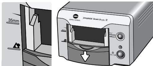
With the scanner contacts face up, insert the adapter into the scanner until it stops. The scanner detects the holder and automatically loads the film. Do not remove the holder until the film has been rewound, see page 21.
