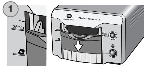
Insert the film holder into the scanner in the direction indicated by the arrow. Hold the holder straight and level with the orientation indicator up (2).
