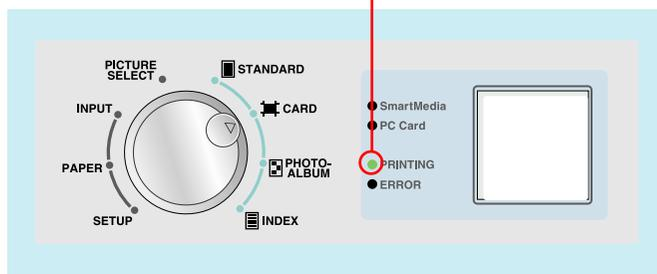
The lamp flashes when the PRINT button is pressed after which printing begins.
