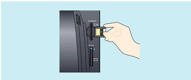
Insert SmartMedia all the way into the printer.
