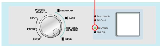
The lamp flashes when the PRINT button is pressed after which printing begins.
