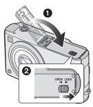
If the card/battery door cannot be completely closed, remove the card and insert it again.
