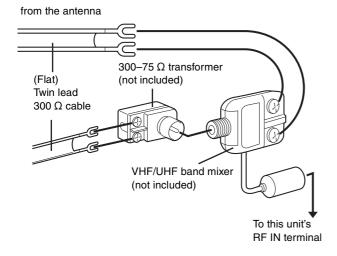
If your television has both lead and coaxial VHF terminals, use the lead connection to minimize signal loss.
