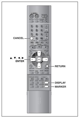
You can mark positions by pressing [MARKER]. Also use on-screen menus to mark, recall, and clear positions.
