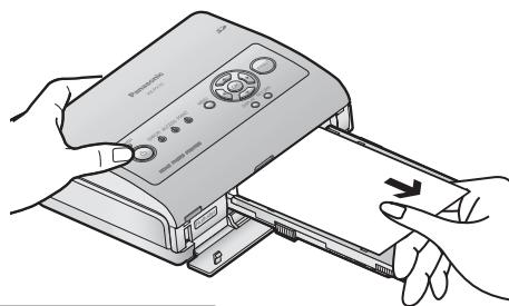
**2 Remove the paper from the front panel ① or rear panel ②.**
