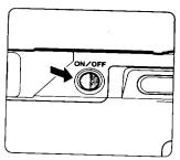
When the main switch button is depressed, the power turns ON.
