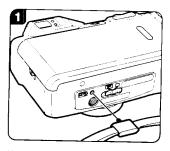
If you wish to unload a film before exposing all the frames, push the mid-roll rewind button with the protrusion part of the strap clamp; the lens retracts to the shortest focal length and then film rewinding starts.
