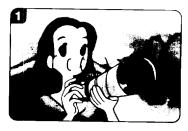
1 When taking a photograph like the one shown above, if the photograph is taken with the camera in this setting, the focus will be placed on the subject in the very front of the (( )) and will not focus on the main subject in the back. In this case, use the Spot AF Mode and focus-lock technique.
