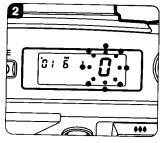
When rewind is completed, the motor stops, and (3) blinks, indicating that the back cover may be opened safely.
