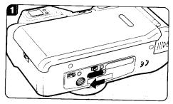
You can switch between the panorama format and standard format picture taking mode at any time by moving the panorama switch. The panorama format picture allows horizontally positioned dynamic pictures to be taken (approx. 13x36mm on film).
