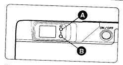
When you depress the shutter release button halfway down, the green lamp and/or red lights up or blinks as shown above.
