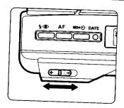
Aim the camera toward a bright subject. While looking through the viewfinder, move the diopter adjustment lever to the right or left until the AF frame appears in the sharpest focus.
