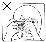
Keep the camera as still as possible, and gently depress the shutter release button. If too much force is applied, the camera is likely to shake, and the picture will be blurred. When using the flash with the camera positioned vertically, hold the camera so that the flash is above the lens.
