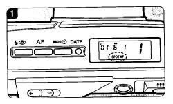
Select the Spot AF Mode to focus on a particular spot in the frame.
