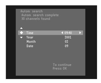
Adjust 'Time', 'Year', 'Month', 'Date' if required, with the  $\nabla$  (down cursor) or  $\triangle$  (up cursor) key. Change values with the the  $\triangleleft$  (left cursor) or  $\triangleright$  (right cursor) key or the digit keys **0-9**. To end, press **OK**.
