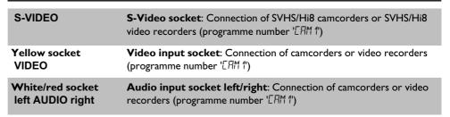
Switching between sockets **S-VIDEO** and **VIDEO** is done automatically. In case both sockets are used, the signal received at socket **S-VIDEO** is treated with priority.
