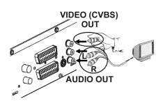
Insert one end of the supplied video (CVBS) cable into the yellow Cinch socket OUT VIDEO (CVBS) at the back of the DVD recorder and the other end into the video input socket (usually yellow) on the TV set (usually labelled 'Video in' or 'AV in'. See TV operating instructions).
