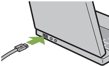
4 Open the terminal cover, and then connect the USB cable to its USB terminal.
