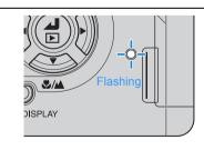
While the camera is accessing the memory card, such as recording images to or reading data from the memory card.
