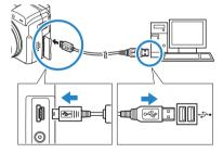
P Important Check the size of the USB connectors. Plug the small connector into the camera and the large connector into the USB port on your Macintosh.
