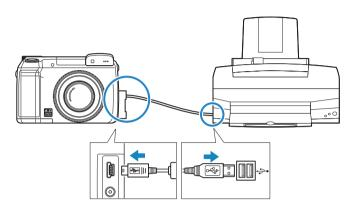
• Important Check the size of the USB connectors. Plug the small connector into the camera and the large connector into the USB port on your printer.
