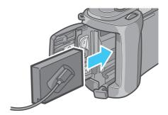
3. Open the power (DC input) cable cover and take the cable out.
