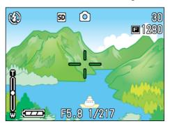
The f-stop (aperture size) and shutter speed are displayed in the bottom part of the screen, and the camera focuses.
