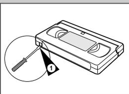
Video cassettes have a safety tab to prevent accidental erasure. When this tab has been removed, you **cannot** record on the tape.
