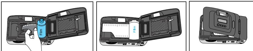
**En** • Open the back cover by sliding the release, as shown above.
