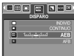
[AFB]: You can select the focus bracket range ( $\pm 1$  step, 3 steps) by rotating the jog dial. Three pictures are taken in a series in different focus range. Use this menu if it is hard to decide distance of the object.
