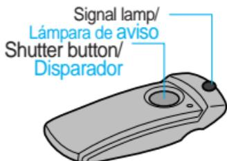
**Names of parts of the Remote Control
