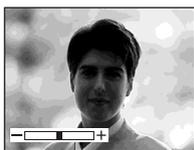
While exposure is set to manual mode,  $\pm$  is displayed in the left-hand corner of the screen.
