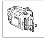
Slide the card cover bar lock downward (a) and open the card cover (b).
