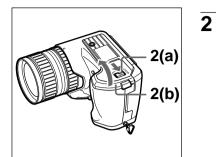
Slide the battery cover lock in the direction of the  $\blacktriangle$  mark (a), and open the battery cover (b).
