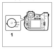
Make sure the camera power/mode dial is set to the OFF position.
