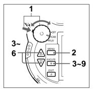
While pressing the mode lock (green), turn the power/mode dial to CAM.
