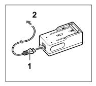
Connect the AC power cable to the battery charger.
