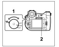
While pressing the mode lock (green), turn the power/mode dial to CAM.
