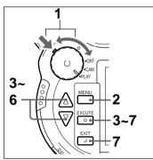
While pressing the mode lock (green), rotate the power/mode dial to PLAY.
