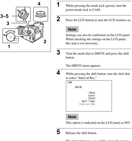
The interval time is set, and the menu disappears. When you press the release button, interval shooting starts.
