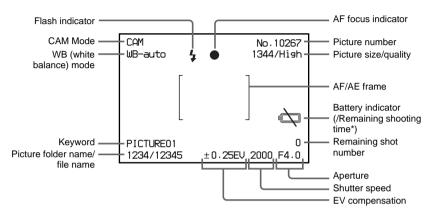
\* Remaining shooting time is not displayed when using AC power adaptor/charger AC-V700. Usually the remaining shooting time is displayed. When the battery gets weak, the battery indicator flashes.
