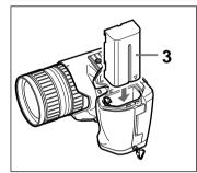
Insert the battery  $\blacktriangle$  mark side first until it firmly locks in place.
