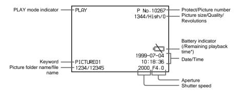
\* Usually remaining playback time is displayed. When the battery gets weak, the battery indicator flashes.
