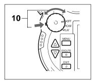
**10** Turning the power/mode dial to OFF turns the power off.
