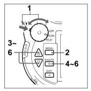
While pressing the mode lock (green), turn the power/mode dial to CAM.
