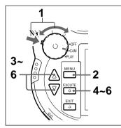
While pressing the mode lock (green), turn the power/mode dial to CAM.
