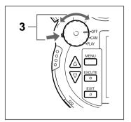
Turn the power/mode dial to OFF to turn off the power.
