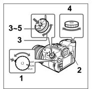
While pressing the mode lock (green), turn the power/mode dial to CAM mode. 2 Press the LCD button to turn on the LCD monitor. Note Settings can also be confirmed on the LCD panel. When checking the settings on the LCD panel, this step is not necessary. 3 Turn the mode dial to USER and then press the shift button. The USER FILE menu appears. 4 While pressing the shift button, turn the shift dial to choose NO. 0 (reset). CAM USER FILE No.0 (reset) 1999-07-04 No.1 No.2 1999-07-04 No.3 1999-07-04
