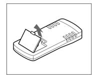
Slide the battery cover in the direction of the ▲ mark while pushing the cover.
