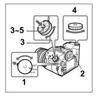
While pressing the mode lock (green), turn the power/mode dial to CAM mode.
