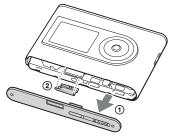
Slide the side part (①) and remove the two screws (②) on the side of this player.
