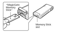
When the "Memory Stick" is inserted into the slot, "ACCESS" appears.
