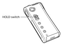
Slide the HOLD switch in the direction of the arrow.
