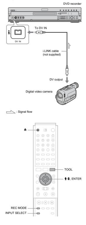
**1** Turn on your TV and this recorder, then set the TV to the connected channel ("VIDEO" etc.).
