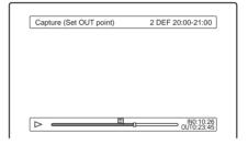
While watching the playback picture, select the end point of the scene using ▷, II, and <</li>
