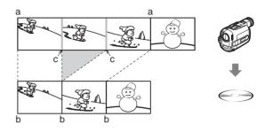
When using a DVD-RW (VR mode), chapter marks [b] are marked where the recordings start on the tape [a]. Chapter marks are also inserted at the IN points of the selected scenes [c]. For other discs, the recorder marks chapters either in 6 or 15 minute intervals depending on the setting in "Auto Chapter" in Features Setup (*page 79*).
