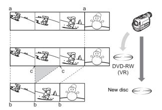
When dubbing to a DVD-RW (VR mode), chapter marks [b] are marked where the recordings start on the tape [a]. Chapter marks are also inserted at the IN points of the selected scenes [c].
