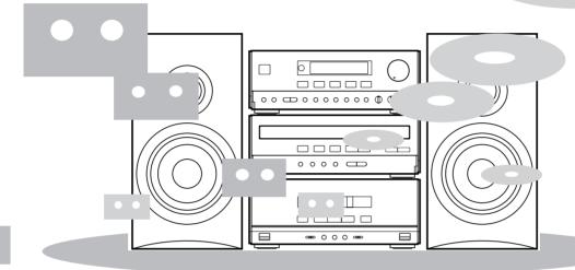
CC-70W is composed of RX-S70, CDC-S90, KXW-S70 and NX-S70. CC-70S is composed of RX-S70, CDC-S90, KX-S90 and NX-S70. \* For U.K. and Europe models, NX-S70 is optional in some areas.
