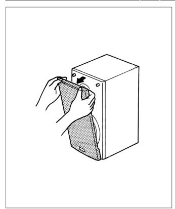
The front grille is fastened to the enclosure at four points, and can be removed if desired. To remove the grille, hold on to both sides and slowly pull straight away from the speaker. To reattach, line up the four pegs on the speaker with the four corresponding holes on the inside surface of the grille and push gently.
