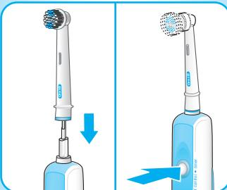
Attach one of the brushheads (1 or 2) to the handle. You can use any kind of toothpaste. To avoid splashing, guide the brushhead to your teeth before switching the appliance on.
