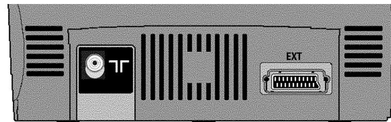
**T** **Aerial input socket:** To connect the aerial cable
