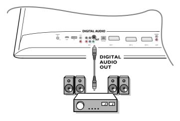
Connect a digital MultiChannel Surround receiver to the DIGITAL AUDIO OUT connector at the bottom of the TV.
