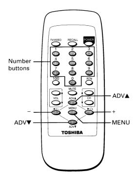
6 Press ADV to lock out the channel.
