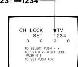
6 Press ADV to lock out the channel. The display at the right will appear on the screen for about 4 seconds.
