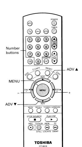
6 Press ADV to lock out the channel. The display at the right will appear on the screen for about 4 seconds.
