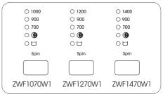
Press the Spin button repeatedly to change the spin speed, if you want your laundry to be spun at a speed different from the one proposed by the appliance.
