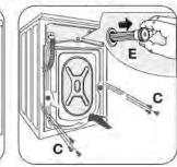
Remove the bracket D, refit the six smaller bolts C and slide out the relevant plastic spacer E.
