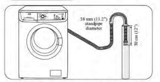
Firstly form a hook in the end of the drain hose using the «U» piece supplied. Place the drain hose into your standpipe, which should have an internal diameter of approximately 38mm thus ensuring there is an air break between the drain hose and standpipe. When discharging into a standpipe ensure that the top of the standpipe is no more than 90 cm (35.4") and no less than 60 cm (23.6") above floor level.
