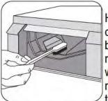
Having removed the drawer, use a small brush to clean the recess, ensuring that all washing powder residue is removed from the upper and lower
