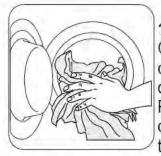
1. Load the laundry Open the door by carefully pulling the door handle outwards. Place the laundry in the drum, one item at a time, shaking them out
