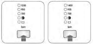
Press the Spin button repeatedly to change the spin speed, if you want your laundry to be spun at a speed different from the one proposed by the appliance.
