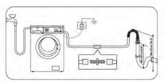
The drain hose may be extended to a maximum of 4 metres. An additional drain hose and joining piece is available from your local Service Force Centre. The joining piece must have an internal diameter of 18mm.
