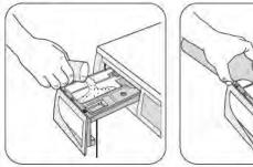
Pull out the dispenser drawer until it stops. Measure out the amount of detergent required, pour it into the main wash compartment L and, if you wish to carry out a programme with the prewash phase, pour it into the compartment marked L
