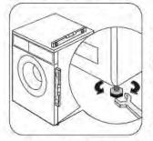
Any necessary adjustment can be made with a spanner. Accurate levelling prevents vibration, noise and displacement of the
